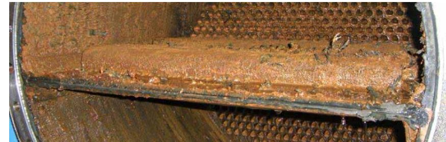
The deposit and accumulation of sludge inside a heat exchanger increases its energy consumption and reduces its performance.
