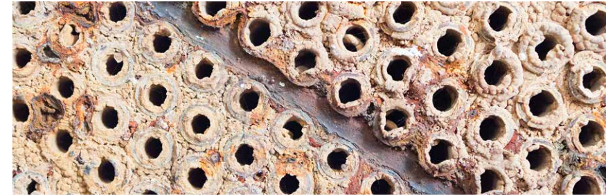
Precipitation of calcium carbonate salts and the presence of corrosion on the heat transfer surfaces of a tubular heat exchanger.
